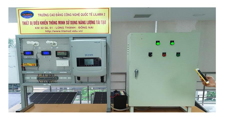
Designed and installed by \_ILAMA 2 teachers: Practical model of multipurpose intelligent electricity with IoT application, integrated with renewable electricity for remote controlling and monitoring
