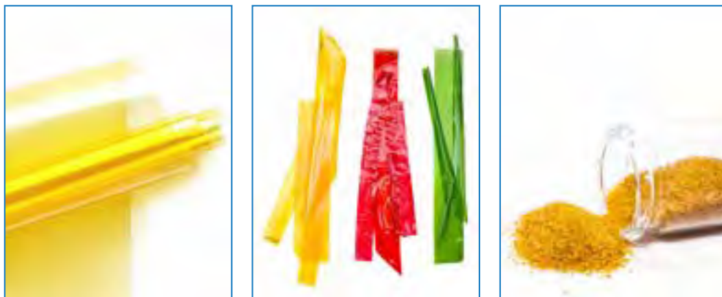
Figure 33: Traceless materials: Film samples, colour film samples and Plast granulates (Source: traceless.eu)
