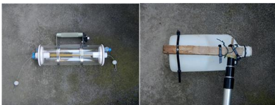
Figure 6-3. Van Dorn water sampler (left) and simple water sampling bottle (right) suitable for water quality sampling in rivers
