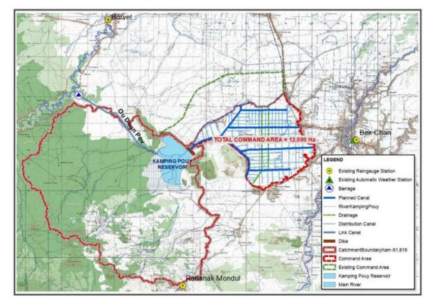
Figure 1: General layout of the Kamping Puoy Irrigation Subproject<sup>1</sup>
