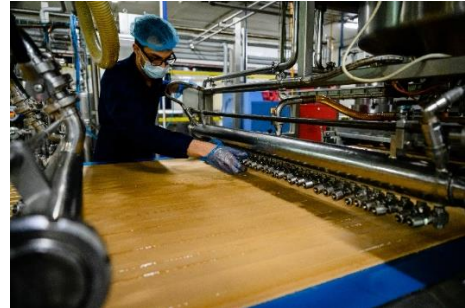
Ammar, a filling line technician at Jordina, calibrating the syrup nozzles.
