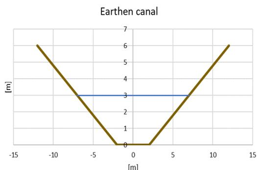
With the estimated canal geometry and an assumption of 3 m water depth in the canal, the total volume along the 15 km is approximately 400 000 m<sup>3</sup>, which is already a considerable water storage.
