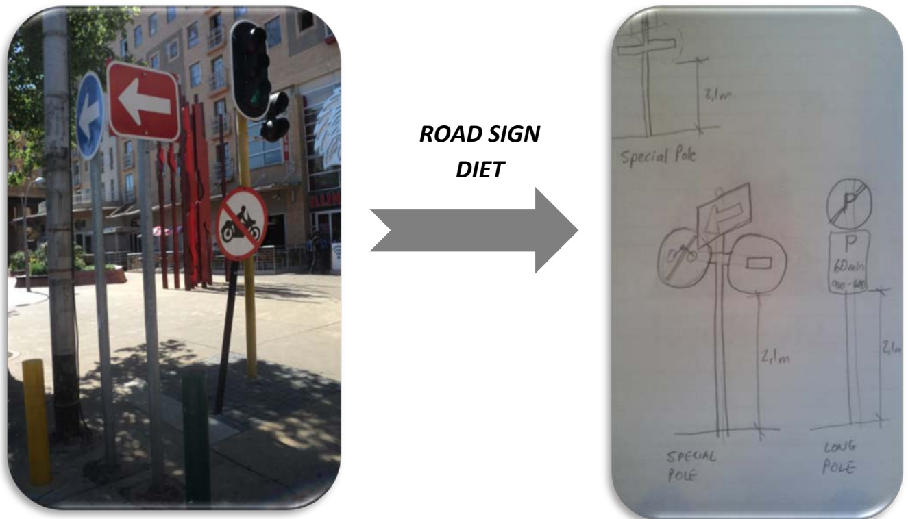
Figure 5-21: Application of a road sign diet
