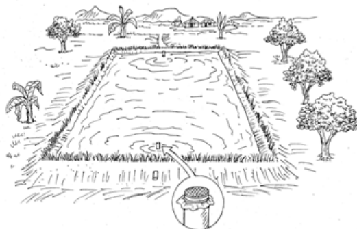
Fig 3.38 screen rightly fixed on overflow
