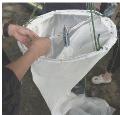
Figure 20. Picture of the microplastic sampling net used in the COMPOSE project in several lakes in Northern Viet Nam.
