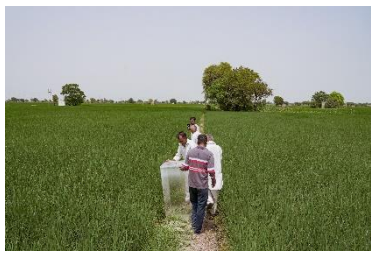
Static gas chamber for GHG sampling: Rice fields in Haryana ©Olam Agri
