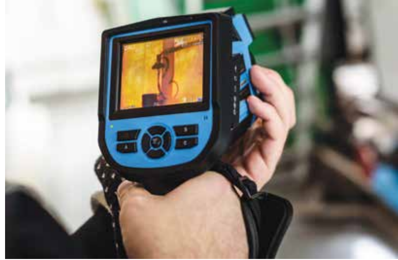
Checking the energy consumption with a thermograph
