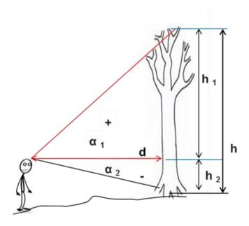
• If the **eye level lies under the ground level**, the angle  $\alpha_2$  (ground reading) is **positive** and the total height (m) is calculated as follows:
