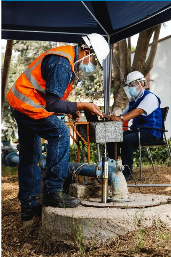
Groundwater monitoring with a probe at the water utility company Sedalib.
