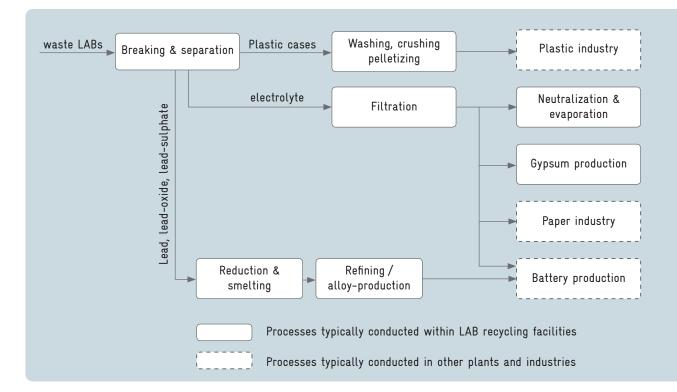
Figure 3/2: Generic flowchart of lead-acid battery recycling Source: Öko-Institut e. V.
