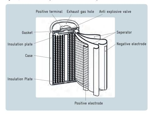
Figure 3/4: Structure of a cyclindrical Lithium-ion battery cell Source: Panasonic 2007
