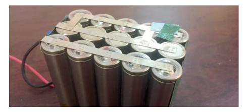
Typical arrangement of Li-ion cells for a battery pack used in SHS © Öko-Institut e.V. There is an intensive debate on differences in fire safety of different types of Li-ion batteries. These debates usually refer to the following aspects:
