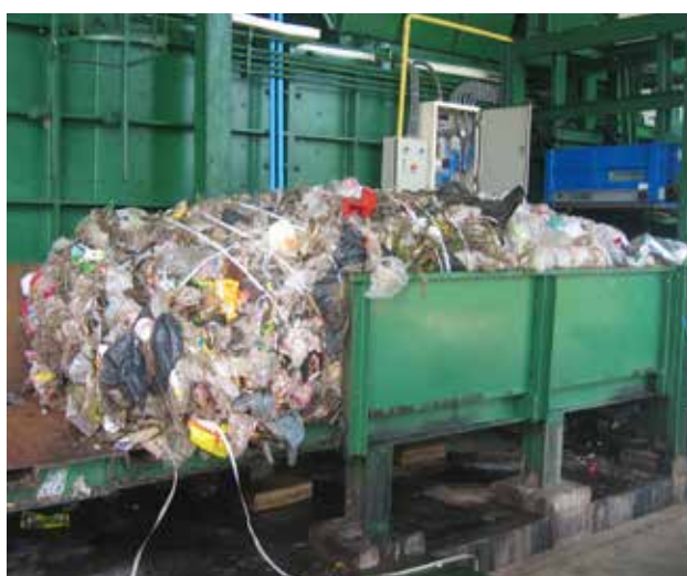
Compaction of sorted plastic waste in Fang Municipality, Thailand
