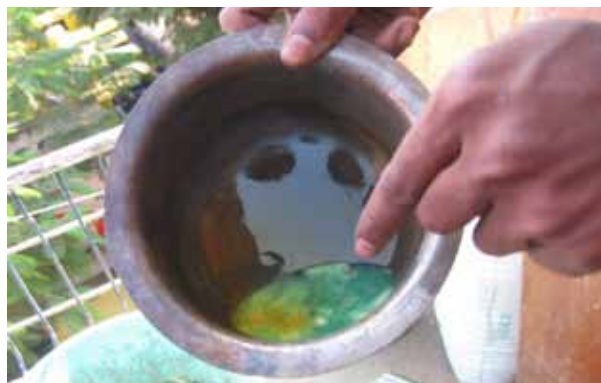
Worst Practice: Leaching of PWBs ©Empa
