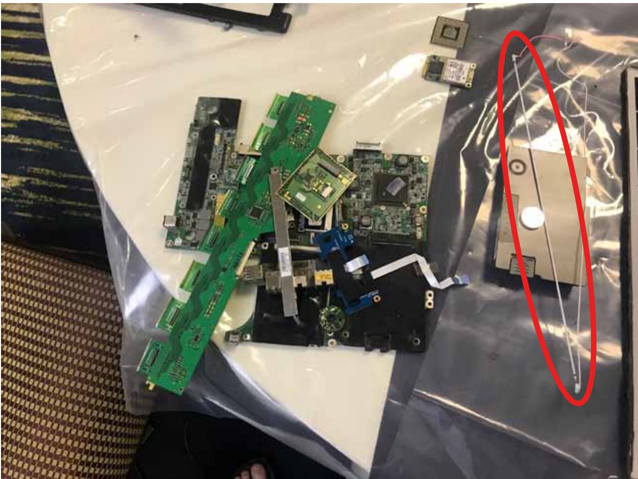
Figure 2: Fluorescent Lamp found in laptop screen which has high concentrations of mercury (Courtesy of Reclite SA (Pty) Ltd)
