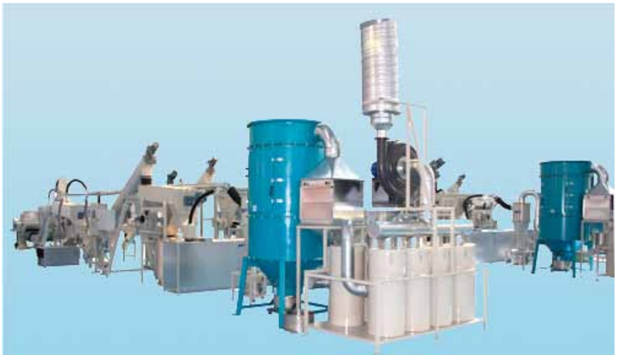
Figure 4: Lamp processing plant (Courtesy MRT, Sweden)
