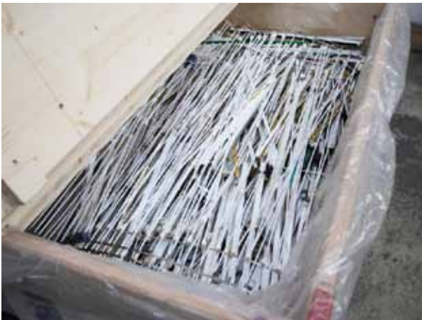
Safe storage in a box (with cover) for undamaged fluorescent tubes in a safe way
