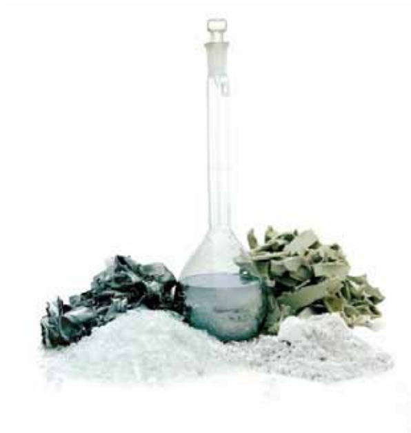
Figure 5: Recovered fractions from the lamp processing plant (Courtesy Reclite SA (Pty) Ltd)
