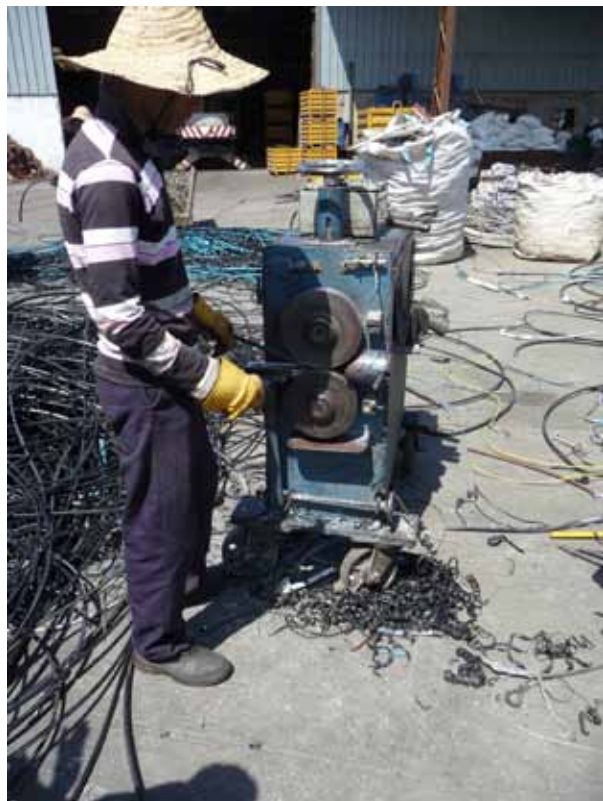
Good Practice: Cable stripper avoiding air pollution ©Empa
