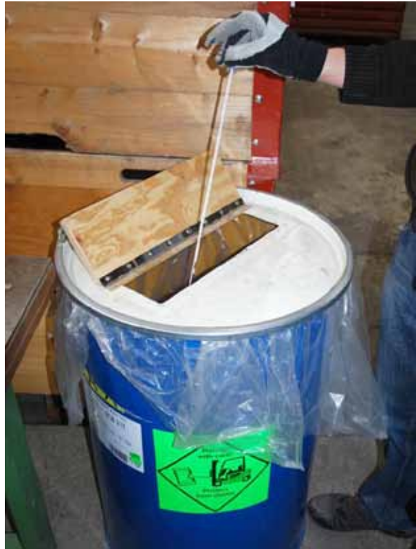
Barrel with a special cover to store broken fluorescent tubes in a safe way
