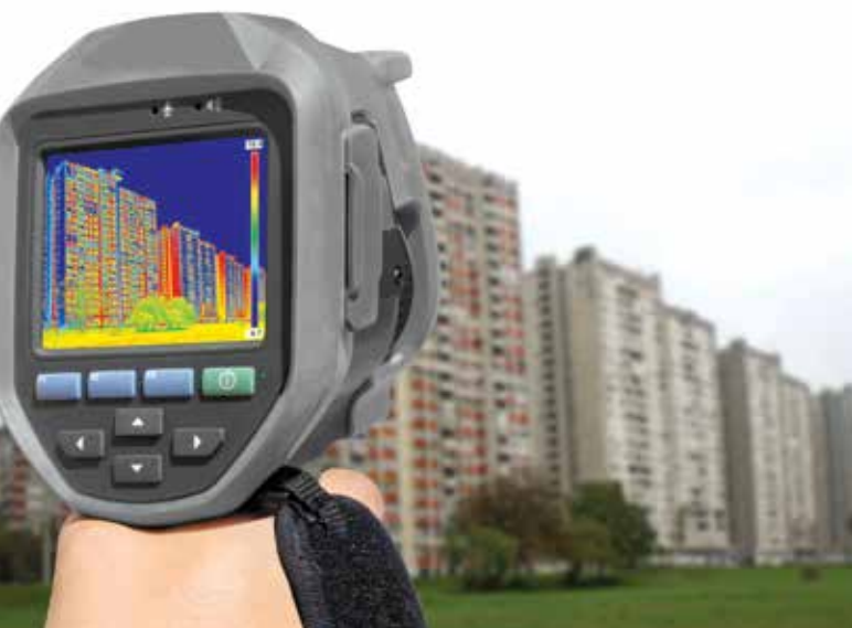
Recording heat loss using an infrared thermal camera
