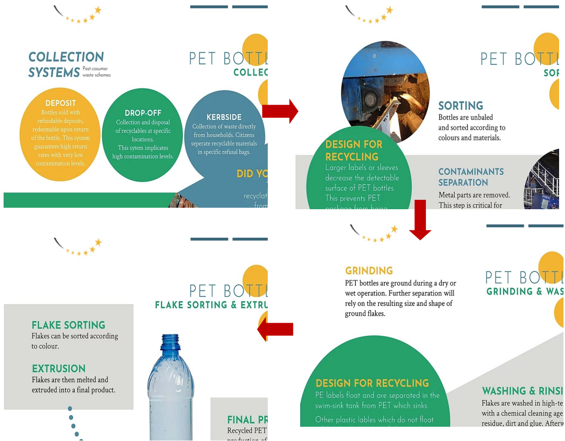
Figure 3: PET bottle-to-bottle recycling process (Source: https://www.plasticsrecyclers.eu/how-does-recycling-work )
