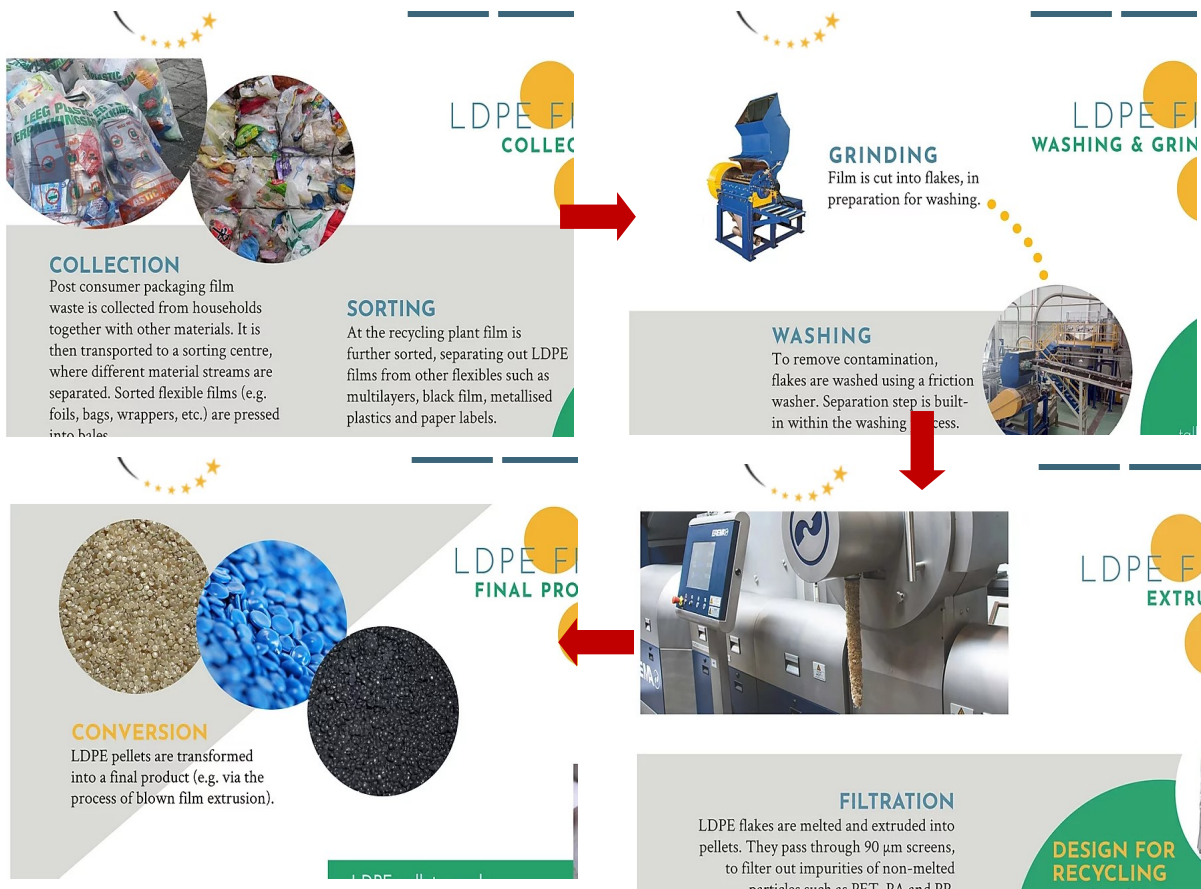
Figure 4: LDPE film recycling process (Source: https://www.plasticsrecyclers.eu/how-does-recycling-work )
