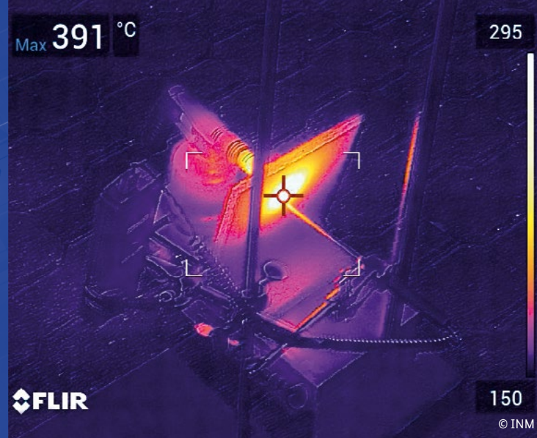
Testing the heat and flame resistance of construction panels made from bush biomass
