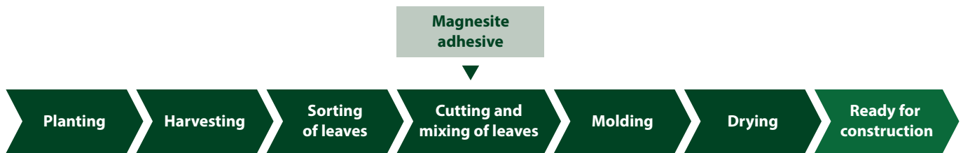
Figure 2 Manufacturing process of typha blocks
