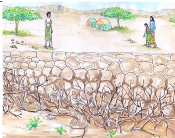
Fig. 7: Organic matter will sediment and water infiltrates, enriching the land above and below the drystone structure
