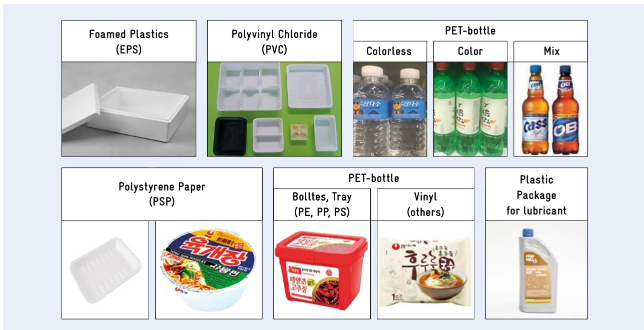
Figure 14: Examples of mandatory recycling items for plastic packaging materials by EPR in Korea
