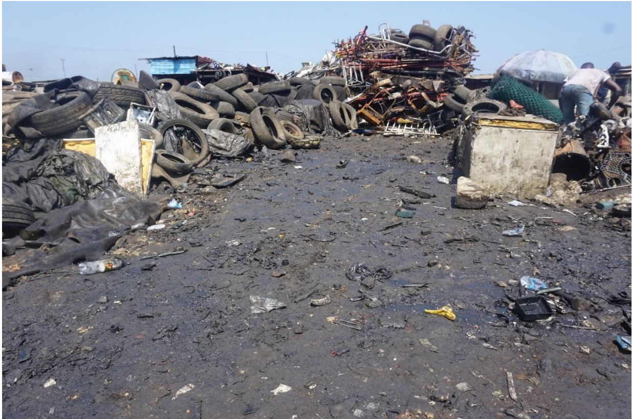
Img.: A car dismantling shop and the harmful remains of the improper manual dismantling process: brake fluids, oil, coolant and fuel have contaminated the ground / ©GIZ
