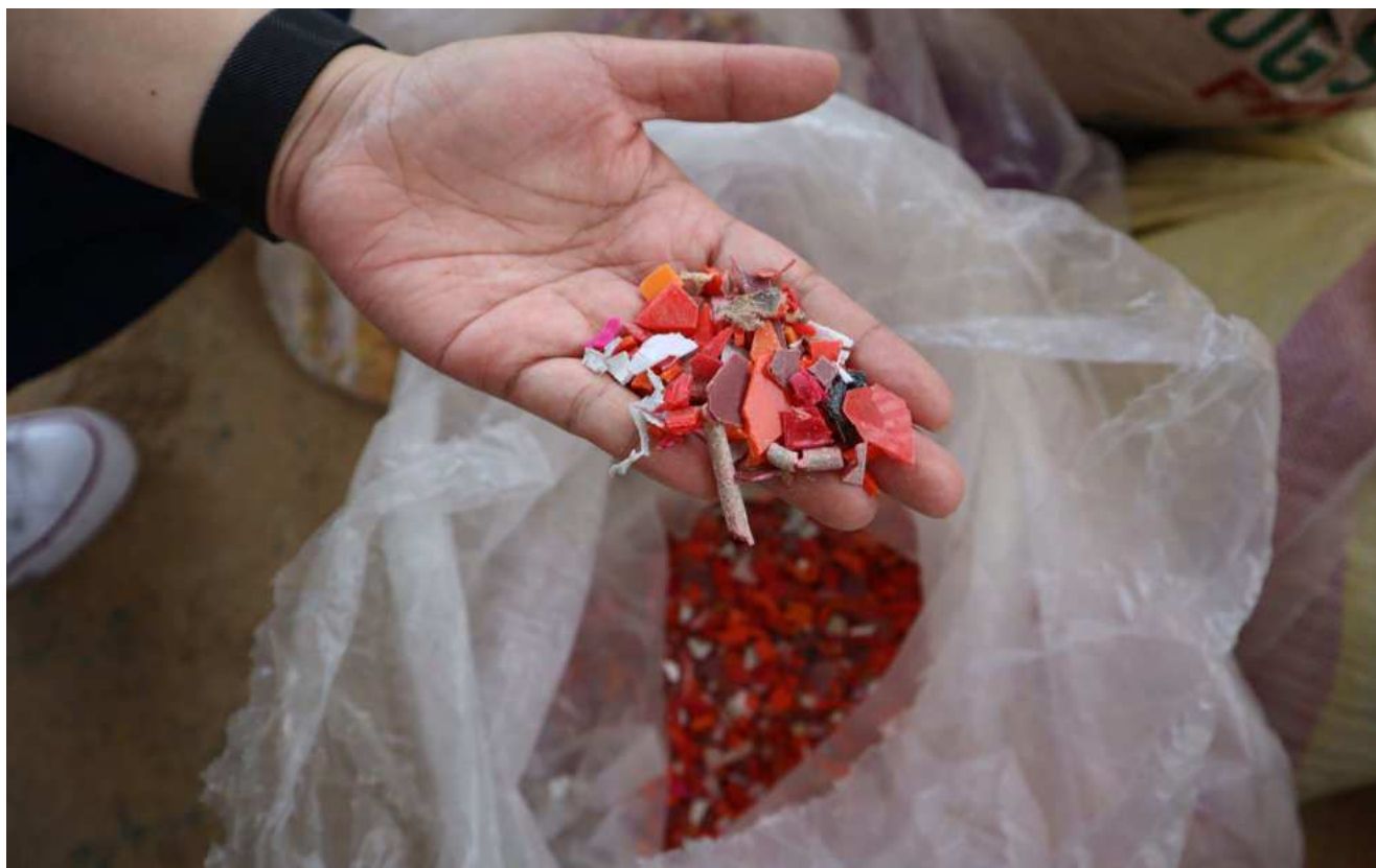
At the Sapal facility donated by DENR, plastics undergo shredding, melting through an extruder, and molding into recycled lumber that can then be used for furniture, construction materials, and other materials.
