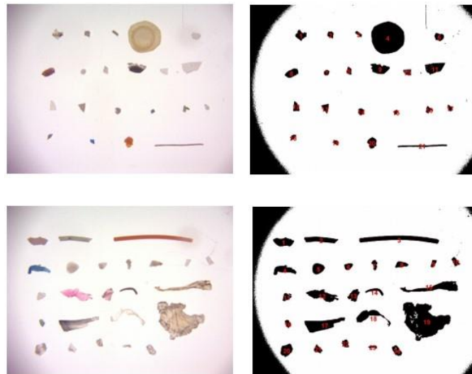
Figure 6.7. Digitally photographed image of particles on petri dish (left) and binary image of numbered particles by image processing software (right)
