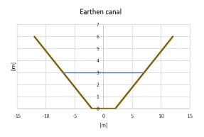
With the estimated canal geometry and an assumption of 3 m water depth in the canal, the total volume along the 15 km is approximately  $400\ 000\ m^3$ , which is already a considerable water storage.
