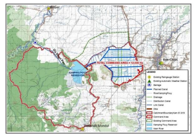
Figure 25: General layout of the Kamping Puoy Irrigation Subproject <sup>13</sup>
