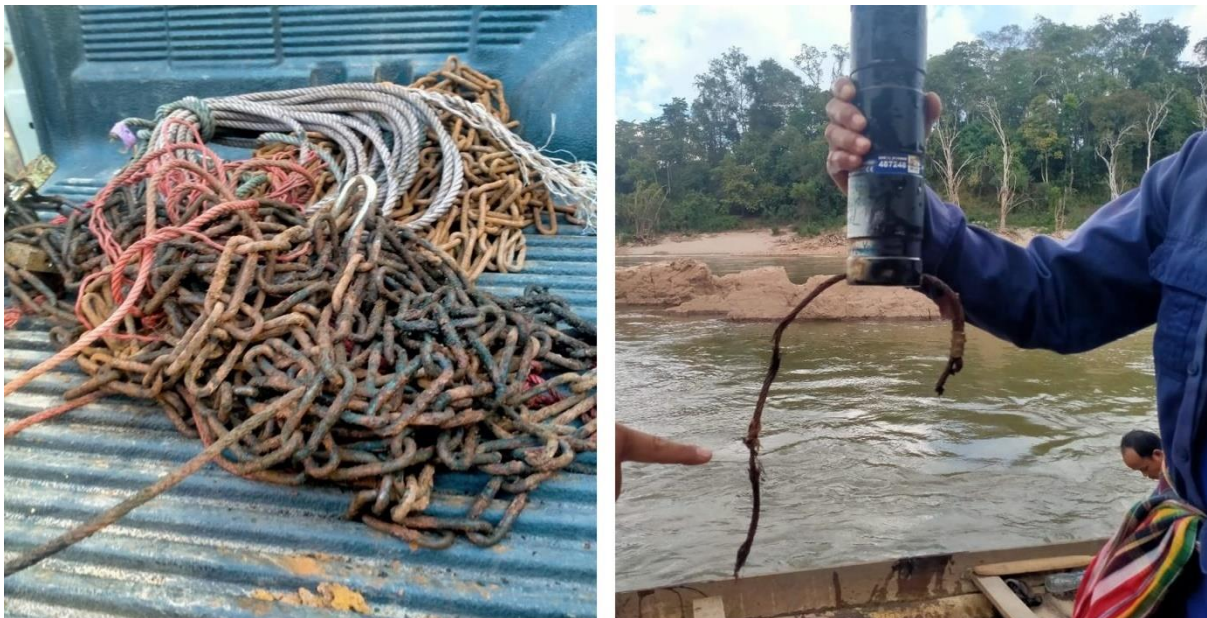
Plate 14. Badly rusted and worn receiver security chains and cables in November 2022, after just 6 months in the river. The receiver cable on the right is worn through in several places. Stainless steel chain and cables were requested but not available.
