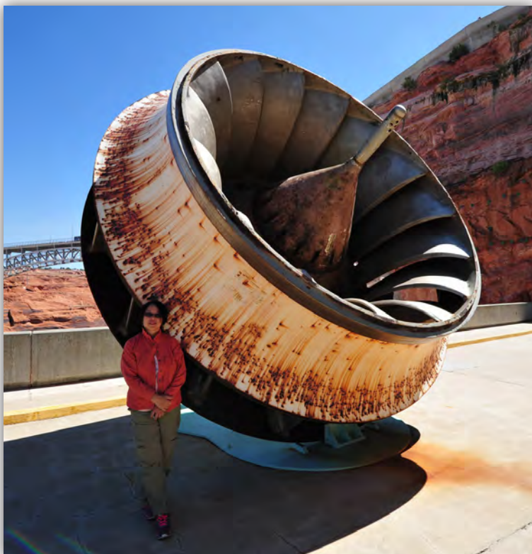
Figure 44: One of the eight original Francis turbine runners from Glen Canyon Dam, Colorado River, USA
