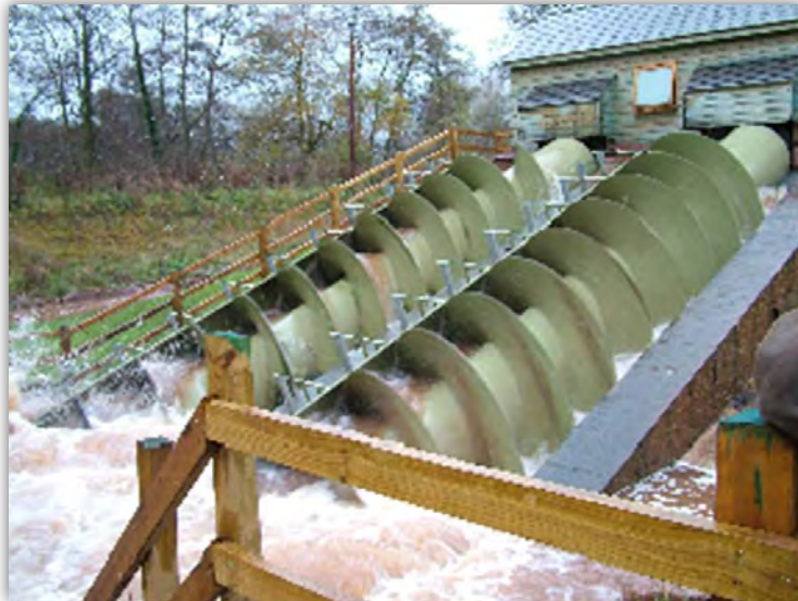
Figure 47: A hydropower turbine being run by an Archimedes screw, an ancient design
