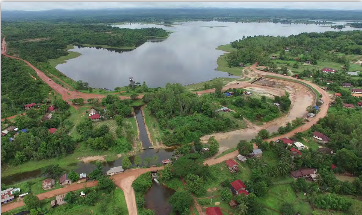
Figure 9: Nam Souang, a typical shallow irrigation reservoir in the Mekong Basin in Lao PDR
