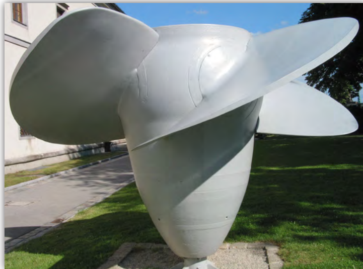
Figure 45: The runner of a typical Kaplan turbine
