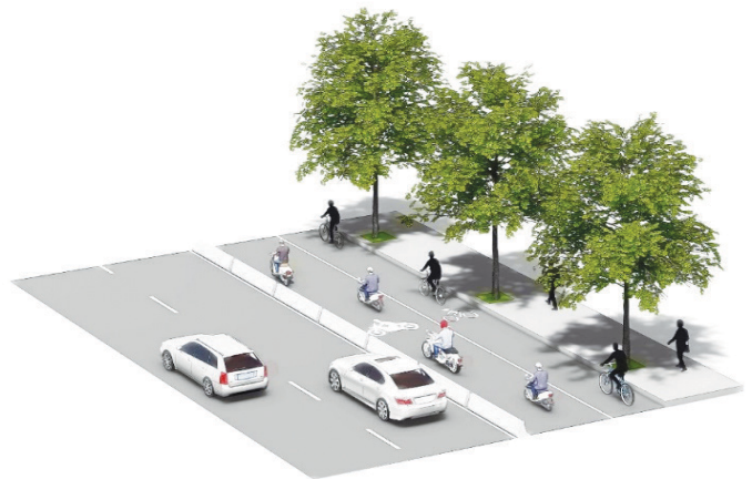
Figure 5.8. Motorcycle lane and bicycle lane are separated by a physical median
