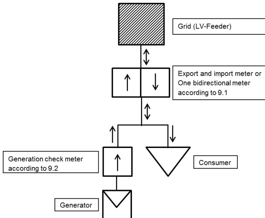
Figure 8: Metering Arrangement
