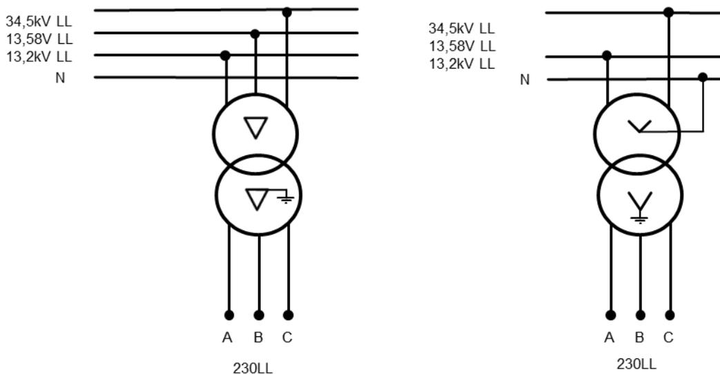
Figure 1: 3-phase-4 wire and 2-phase-3-wire ("three-phase") systems
