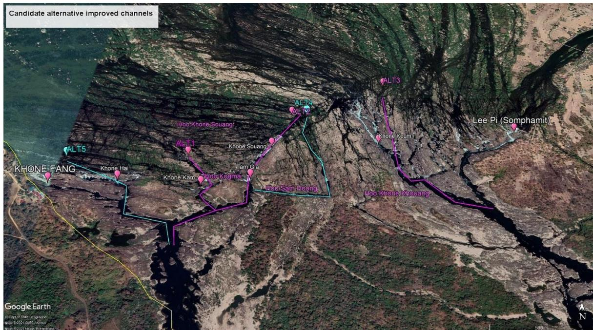
*Figure 4-1. Proposed new channels improvements in Khone Fang area*
