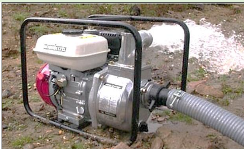
Photo showing a petrol pump connected to the suction pipe operating.
