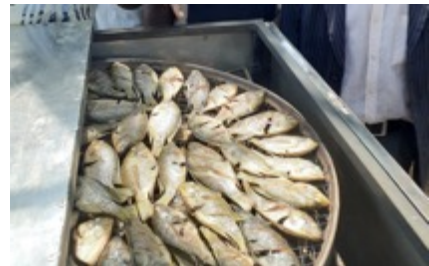
Sliding top cover to monitor progress
