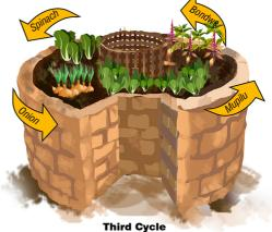
Keyhole gardens made of double layer bricks using a paste of anthill soil paste or a mixture of clay soil, dambo and river sand improves bonding strength than a single layer of bricks with salty antill soil paste. Also making a cement coating layer on top of the Keyhole garden wall, strengthens the structure. However, in future, we intend to construct the KHG using bricks and cement because it lasts longer compared to other KHGs types made of bricks and anthill soil paste.
