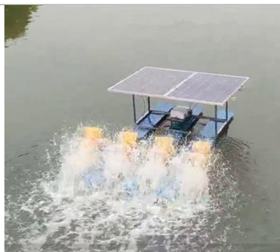
Figure 82: Aeration by solar-powered water wheel
