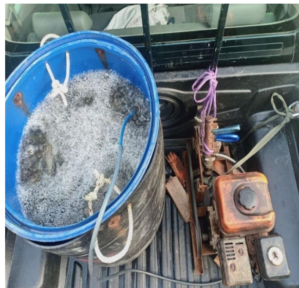
Figure 111: Small tank equipped with a small engine-run aeration system for transporting live fish for longer distances Photo credit: Nen Phanna, SAFR Project
