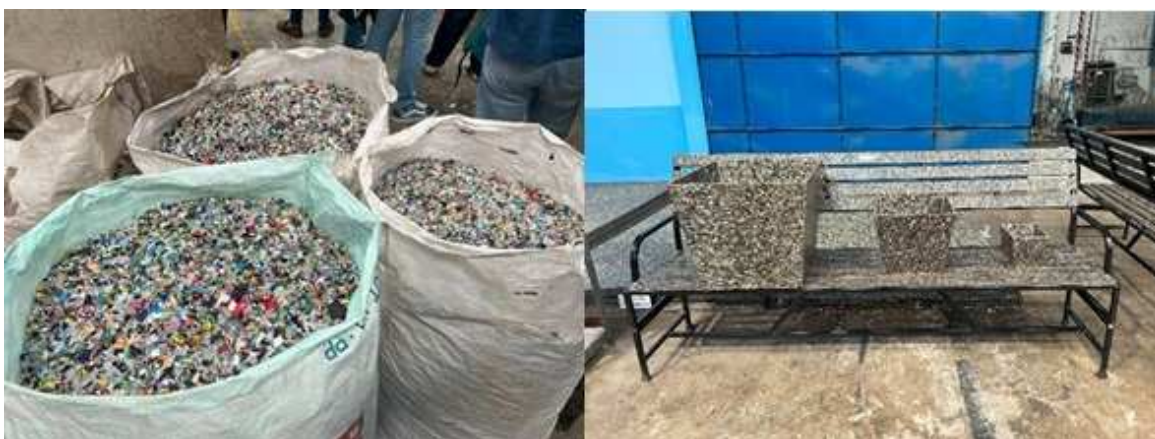
Shredded flexible plastic wastes (left) used in producing benches and plant boxes (right). © GIZ
