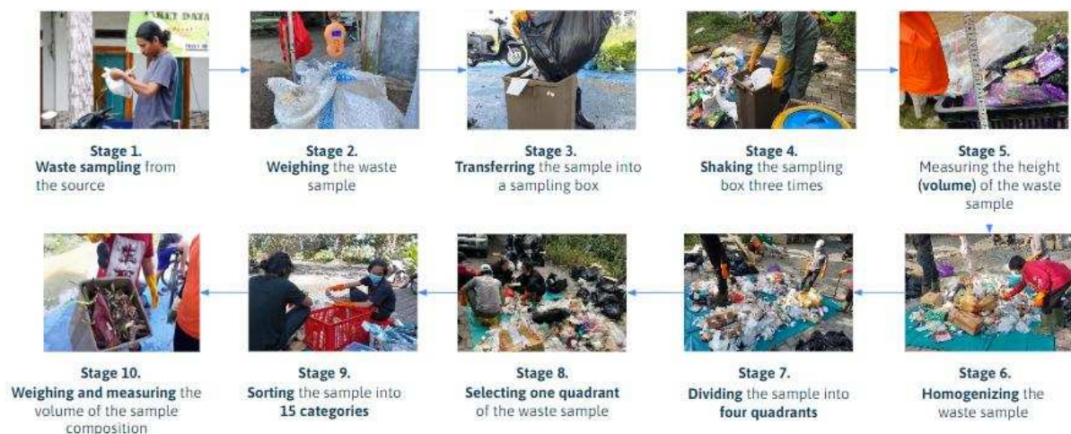
Figure 3.2 Stages of Waste Sampling Activities Based on SNI 19-3964-1994
