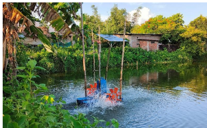
Picture 2: A solar-powered aerator helps fish farmers in Assam to increase the oxygen levels of their ponds. This increases fish and shrimp yield.
