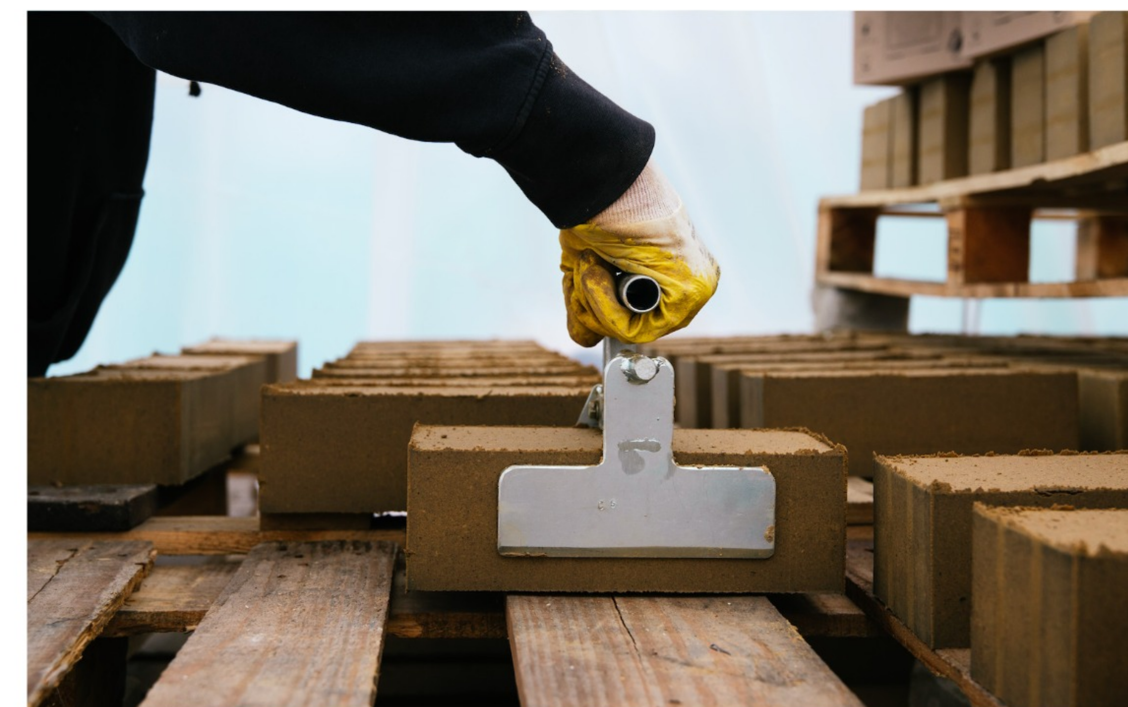
Production of CEBs from local soil in Lviv by Anna Pommazana & Mykhailo Shevchenko. Grunt Experimental Fellowship with Bauhaus Earth. Photo © Zlatozlava Kryshtafovych
