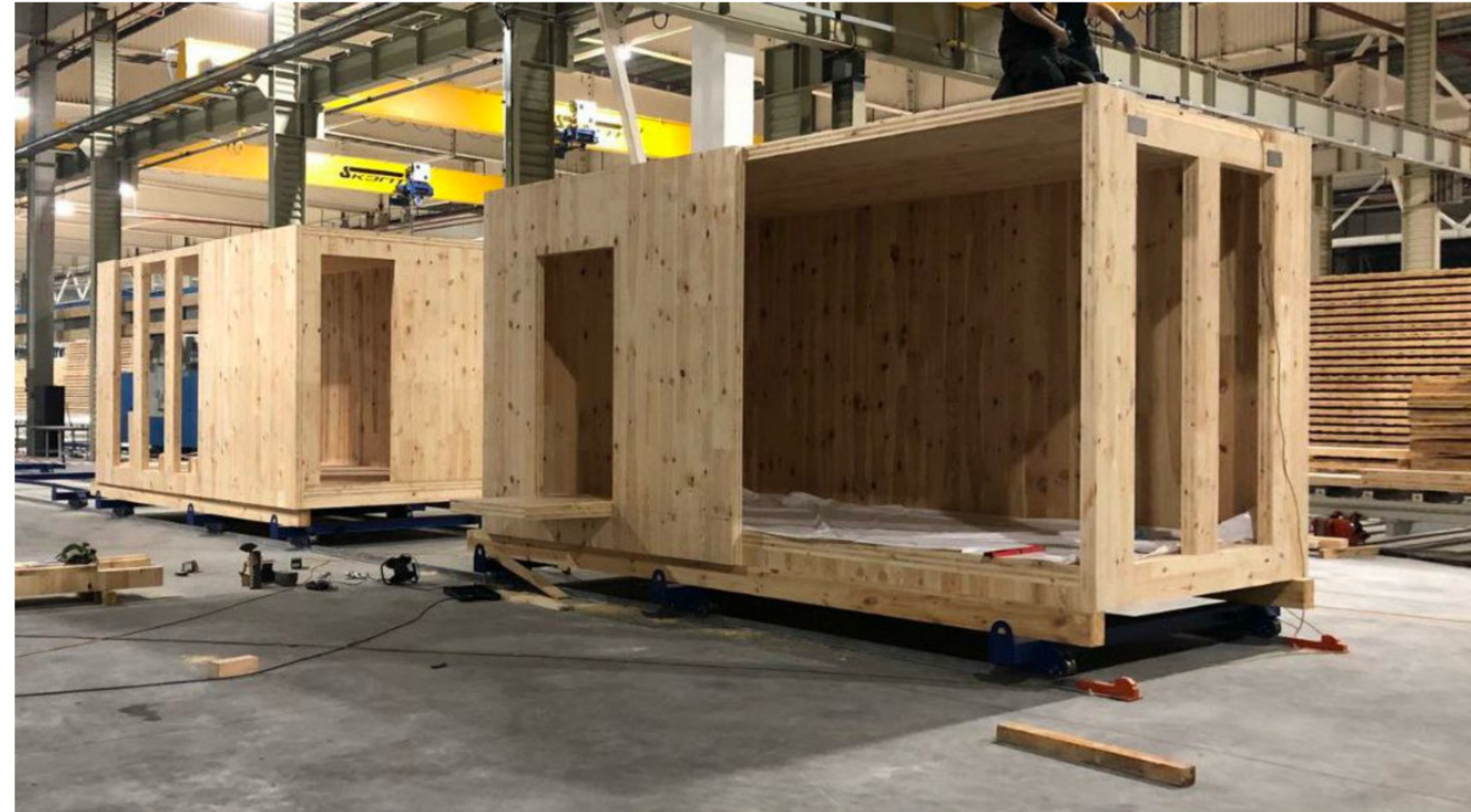
CLT Modules produced in Korosten, Zhytomyr Obl., © CLT Rezult. https://clt-rezult.com/en/
