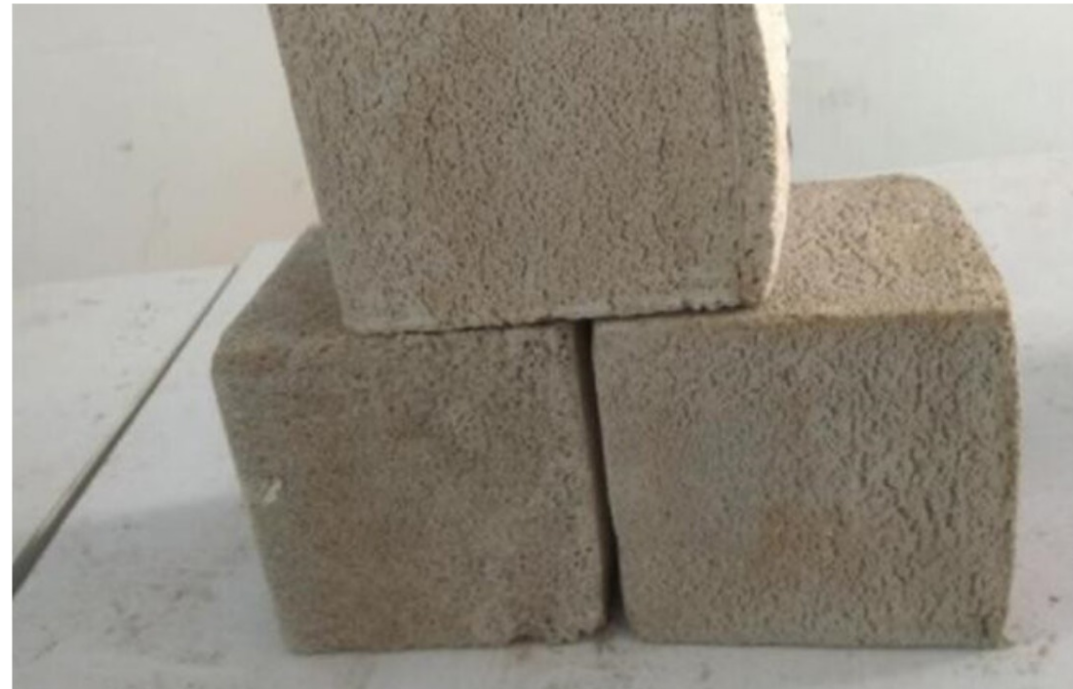
Iron-ore slag foamed concrete block. Photo ©
